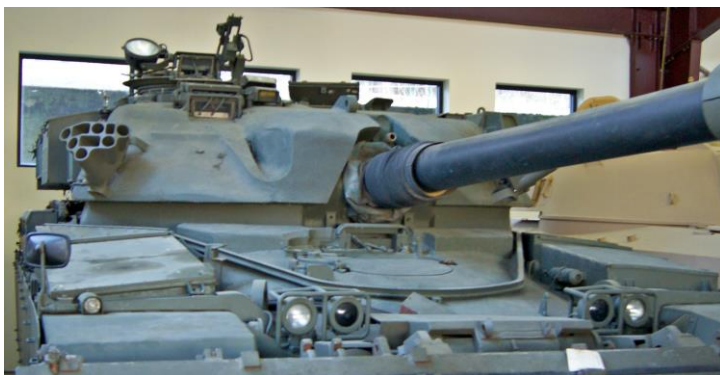
Figure 73: FV4201 Chieftain Main Battle Tank with Stillbrew Crew Protection Package
