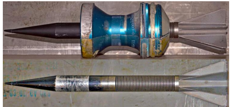
Figure 56: APFSDS Sub-Caliber Penetrator and its Sabot
